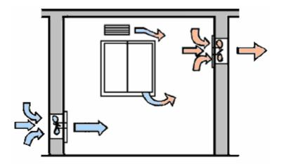
Combined System (Forced Intake & Forced Exhaust)
